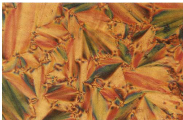
Figure 4. Texture of compound 9 (191°C, on cooling) \times 150.
